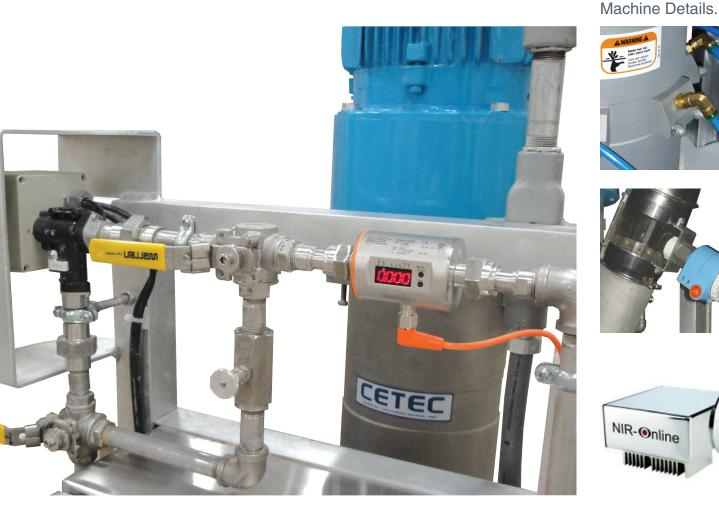
CETEC's HMX Hydromax hydrator is designed to add moisture to finished granulates and powders.
